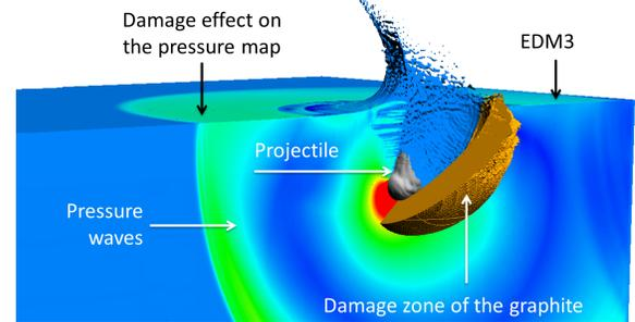
Figure 2: Visualization of the pressure and the damage of a graphite sample with the 45 degrees oblique impact of a steel projectile around 4km/s. The visualization of the 1024 compute engines on TERA takes about 45 seconds. Then the 2048 data files are loaded in about 30 seconds. The computation of the visualization takes less than 5 seconds depending of the algorithms used.
